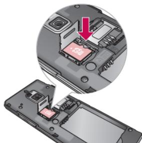
The slot has to be opened by pulling the metal cover upwards.
