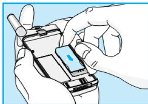
Locate the SIM card socket in the back of the phone.
