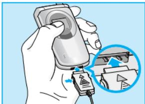
1. Insert one end of the travel adapter into the bottom of the phone.
