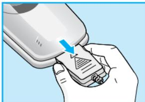
Disconnect the travel adapter from the phone by pressing its side buttons.
