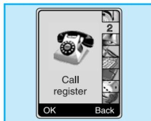
You can check the record of missed, received, and dialled calls only if the network supports the Calling Line identification (CLI) within the service area.
