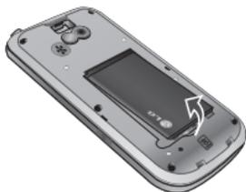
**⚠ WARNING:** Do not remove the battery when the phone is switched on, as this may damage the phone.
