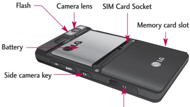
Cable Connector/Battery Charging Connector
