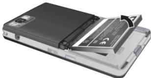
Removing the battery from the phone when the power is on may cause the phone to malfunction.
