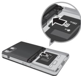
Slide the memory card in with the metal contacts facing down.
