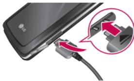
1. With the battery in position in the phone, connect the lead from the travel adapter to the socket on the left side of the phone. Check that the arrow on the lead connector is facing towards the front of the phone.
