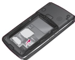
3. Insert the memory card into the slot. The gold contacts must be kept on the back of the microSD memory card. If the memory card doesn't go into the slot easily, you may be trying to insert it in the wrong way or there could be a foreign object in the slot.
