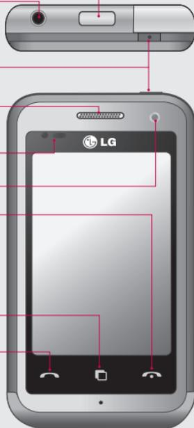
**⚠ WARNING:** Putting a heavy object on the phone or sitting on it can damage its LCD and touch screen functionality. Do not cover the protection film on proximity sensor of LCD. It can be caused the malfunction of sensor.
