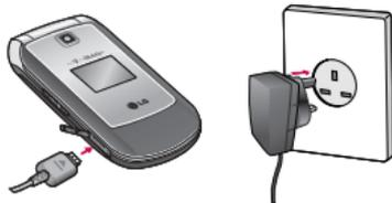
1. With the arrow facing you as shown in the diagram, push the plug on the charger into the connector on the bottom of the phone until it clicks into place.
