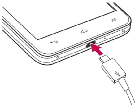
**NOTE:** The battery must be fully charged initially to improve battery lifetime.
