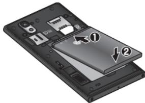
4. Align the back cover over the battery compartment (1) and press it down until it clicks into place (2).
