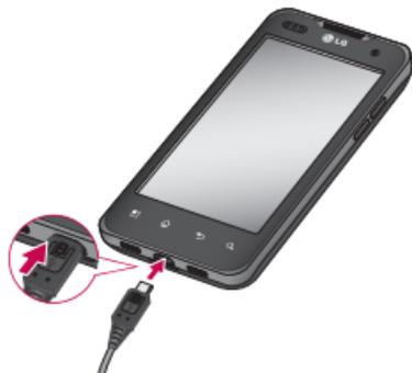
**NOTE:** The battery must be fully charged initially to extend battery lifetime.
