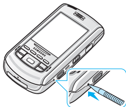
RESET key inside the hole
