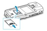
4. Insert the SIM card, ensuring that the cut corner faces top left and the gold contacts of the card face into the phone.
