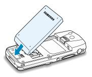
7. Push the battery against the back of the phone until it clicks into place. Make sure that the battery is properly installed before switching on the power.
