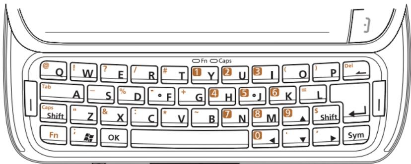
Your Acer M900 Smartphone has a key layout similar to your desktop or notebook computer for greater ease of use. Your Acer M900 Smartphone keyboard also has an embedded numeric keypad (highlighted in orange) for entering number data or dialing phone numbers.
