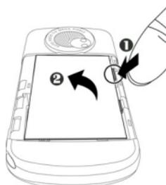
Use the tip of the stylus to carefully unlock the SIM card holder by pushing it down. Lift up the holder and remove the SIM card.
