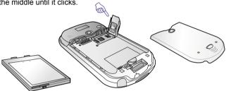
Replace the battery and back cover. Remember to push back the red lock point to clip it into place at the bottom. Push it forward and pull back to secure the SIM.
