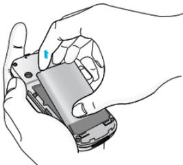
1. Position the lugs on the bottom of the battery into the retaining holder.
