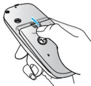
3. Lay the battery cover in place of the phone and slide it until the latch clicks.
