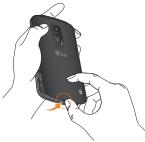
2 Slide the slot protector to the left to unlock it and flip it open. Then insert the microSD card into the slot. Make sure the gold contact area is facing downwards.
