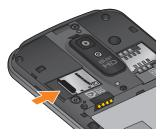
3 Flip the slot protection down to close it. Then slide the slot protection to the right to lock it and replace the battery cover.
