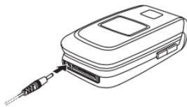
The charging time depends on the charger and the battery used. For example, charging a BL-4C battery with the AC-3 charger takes approximately 2 hours and 12 minutes while the phone is in the standby mode.
