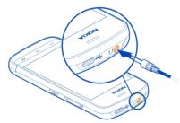
Do not connect products that create an output signal, as this may damage the device. Do not connect any voltage source to the Nokia AV connector. If you connect an external device or headset, other than those approved by Nokia for use with this device, to the Nokia AV connector, pay special attention to volume levels.
