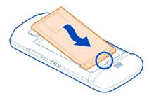
8 To replace the cover, direct the top locking catches toward their slots, and press down until the cover locks into place.
