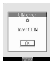
When UIM is missing or damaged
