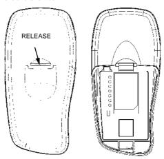
Insert the SIM card into the flap so that the contacts face into the phone, put the sim-card holder flamp back into its seat and lock it with the metal clip. ① Insert the battery so that the connecting cable does not obstruct the battery cover catch, as shown in the figure.
