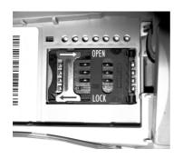
To insert the SIM card, unlock the SIM holder flap by sliding the metal clip in the direction shown by the OPEN arrow.
