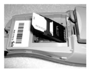
Then lift the flap and insert the SIM card with its contacts facing downwards, as shown here alongside.
