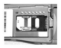
After fully inserting the SIM card, close the flap and lock it with the clip in the direction shown by the LOCK arrow.
