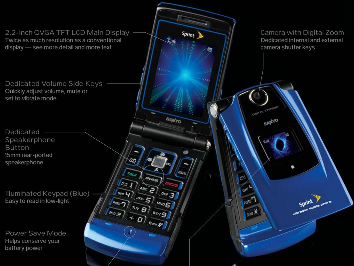
2.2-inch QVGA TFT LCD Main Display
