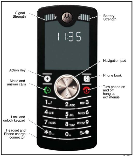
Figure 1. Telephone Controls and Indicators
