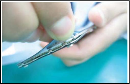
Figure 12. Removing the Keypad Lens
