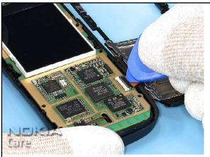
12. Be double careful while opening the connector with the SRT-
