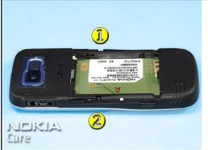
2. Tighten these 2 screws with a torque of 15Ncm, too. Mind the screwing order.
