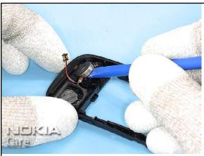
24. Careful lever out the glued in VIBRA MOTOR.
