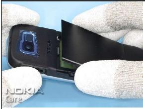
3. Cover all sensitive surfaces with a protective film. Unlock and remove the C-COVER ASSY. Remove the battery if it is still inserted before going on.
