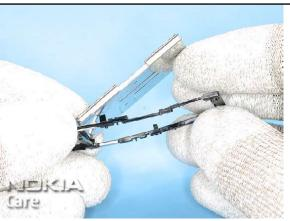
16. Separate the ENGINE SHIELDING ASSY from the C-COVER.
