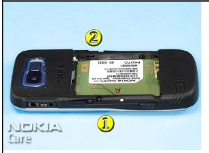
4. Remove both Torx Plus size 4 screws in the order shown.
