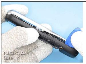
5. Gently pry open the clips of the A-COVER with the SRT-6...
