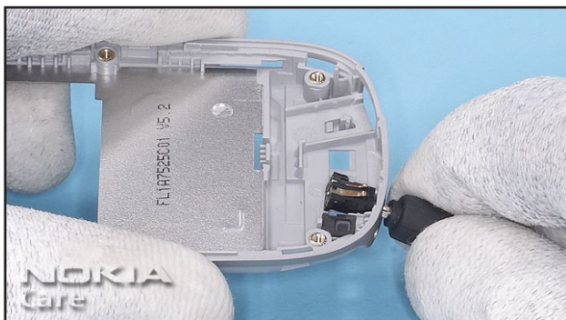
17. Lift out the DC connector with the DC Plug and...
