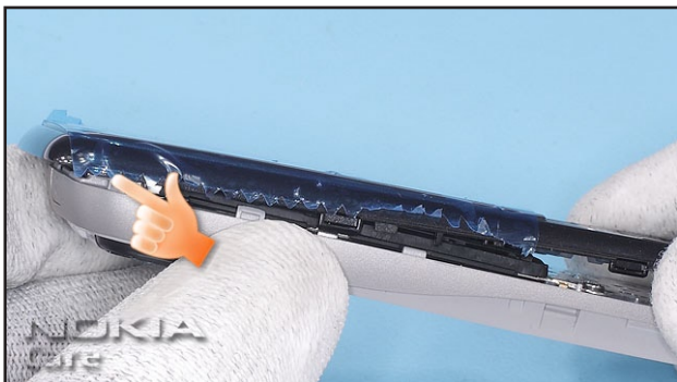
5. Gently lift up the A-COVER ASSEMBLY. Mind the clips on the top.
