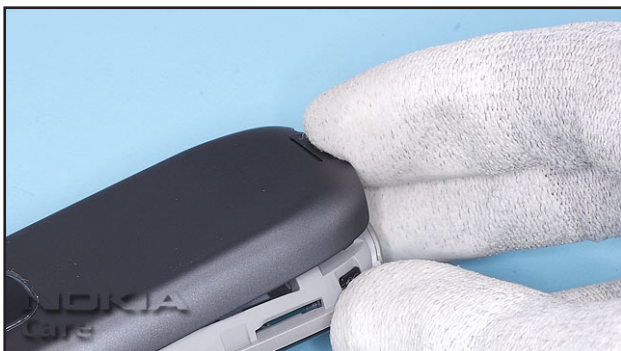
3. Unlock and remove the B-COVER ASSEMBLY.
