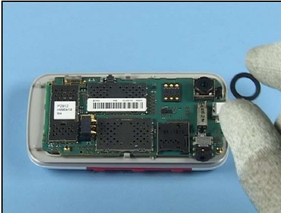
7. Place the CAMERA GASKET.
