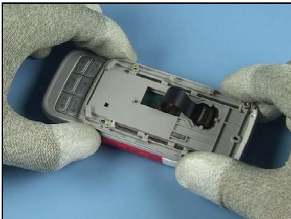
3. Now close the slide mechanism.
