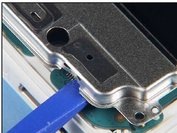
17. After removing the screws carefully disconnect the LCD MODULE connector with the SS-93.
