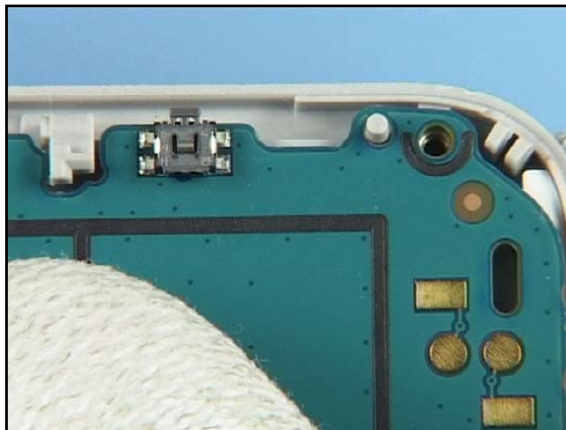
8. Check the position of the UI MODULE again.
