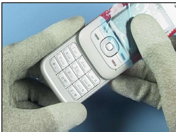
21. At least check the functionality of the slide mechanism.
