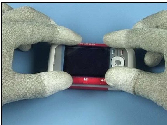
33. Align the A-COVER assembly and push it down evenly. Click all snaps into their places.
