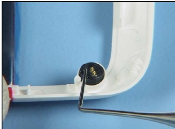
10. Ease out the MICROPHONE with the dental pic.
