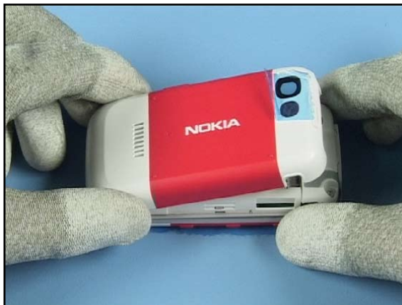
20. Complete the assembly with the B-COVER.
