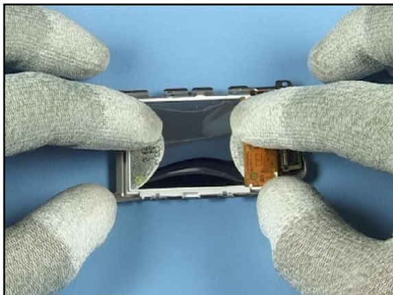
19. Slightly shift down the LCD MODULE as shown.
