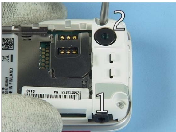
19. Apply the torque to all screws in the order shown.
