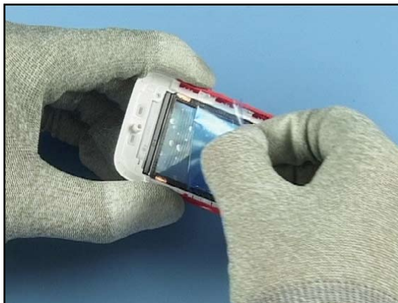
32. Do not forget removing the protective film before continue.
