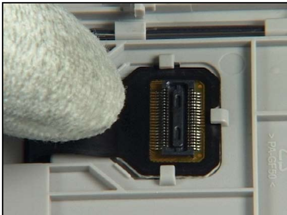
4. Push the connector into position shown.
