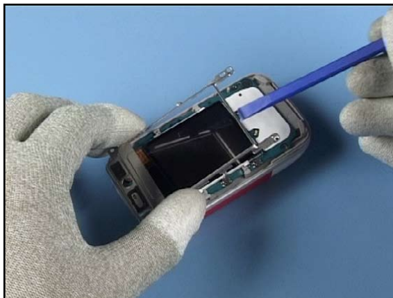
14. Lift up the UI SHIELD assembly.
