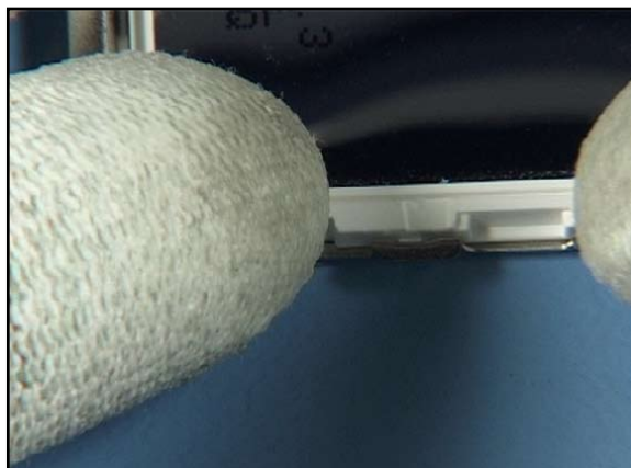
18. Mind the guide while pushing down evenly.
