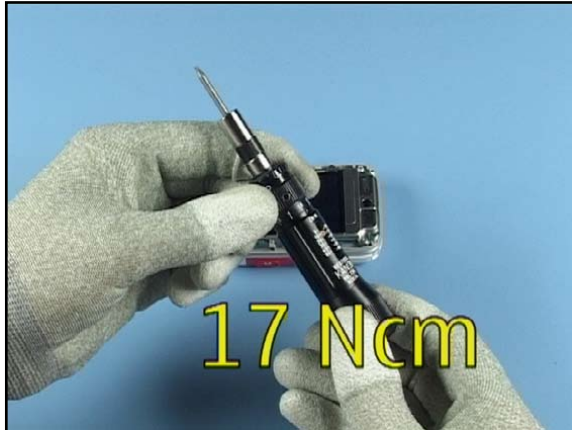
26. Set the correct torque.
