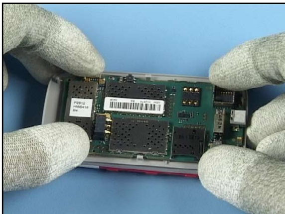
4. Position the ENGINE MODULE correctly.
