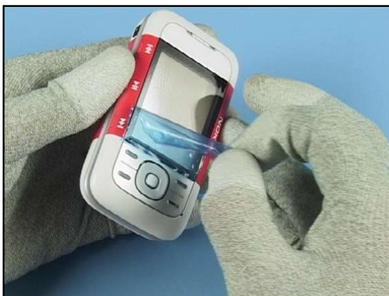
34. Check the window for cleanness.
