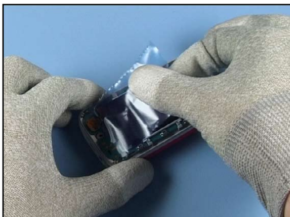
15. Cover the LCD Module with a protective film.
