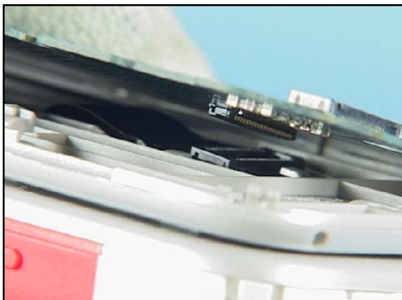
6. Check the positioning of the connector before continue.
