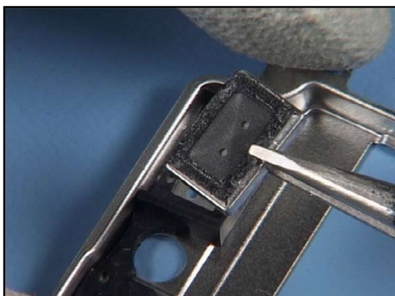
11. Insert the EARPICIE, always fit a new adhesive when replacing the EARPICIE.
