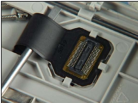
24. Start removing the connector of the SIDE FLEX by lifting it up as shown first.
