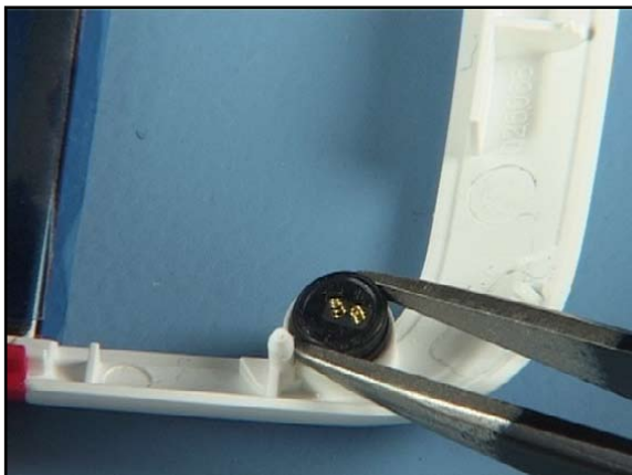
28. Insert the MICROPHONE.
