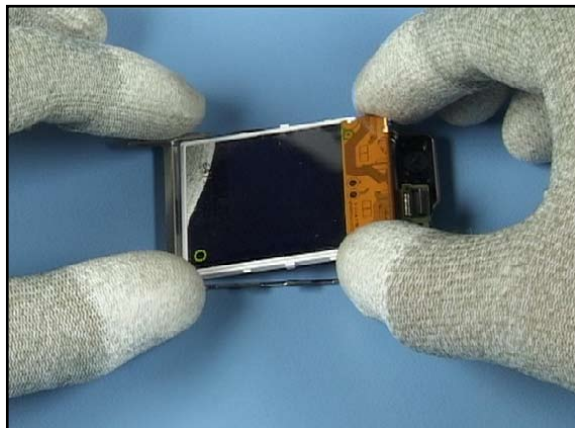
16. Peel up the protection film from the LCD and place it into the UI SHIELD.
