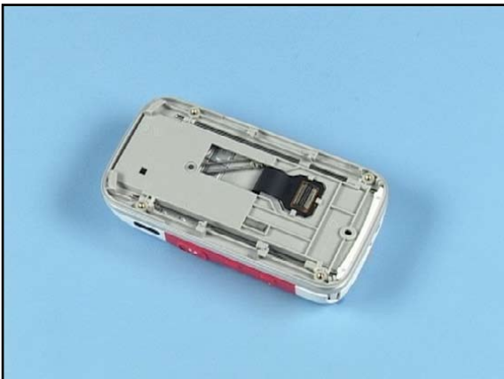
23. To remove the SIDE FLEX both parts of the phone must be disassembled first.
