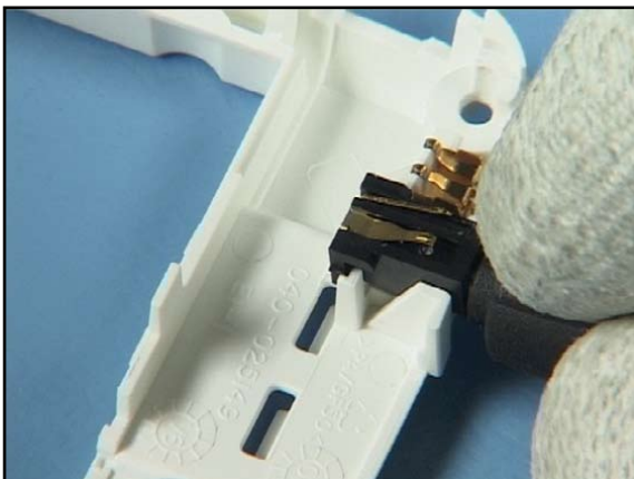
9. Insert the DC JACK with the DC Plug.
