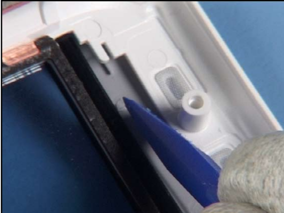
7. The A-COVER DECORATION can now pushed out without the risk of damaging the A-COVER.
