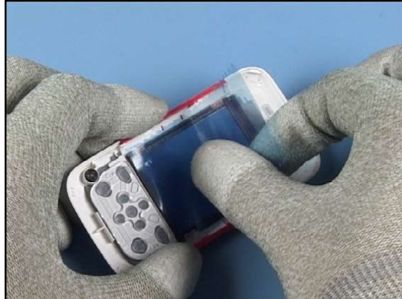
8. Cover the window from inner side with a protective film.
