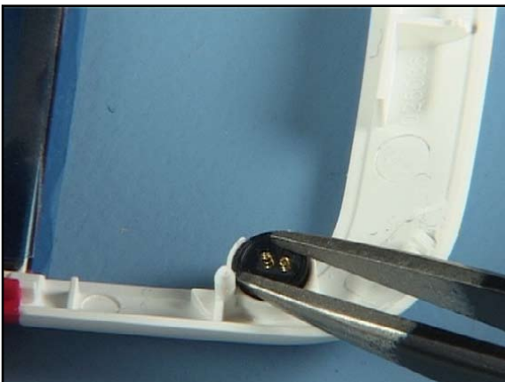
29. Note that the spring contacts are very delicate and can be bent easily.
