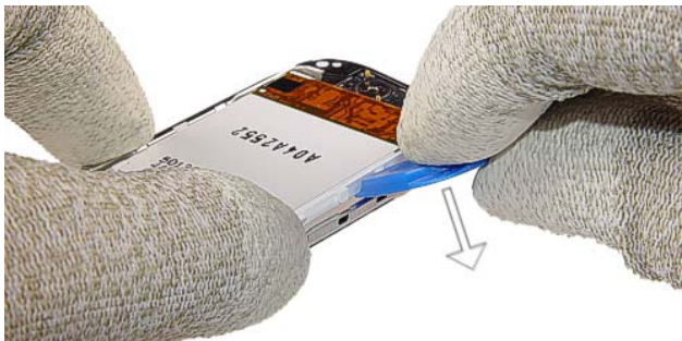
11.) Lever out the LCD Module from the UI Shield .
