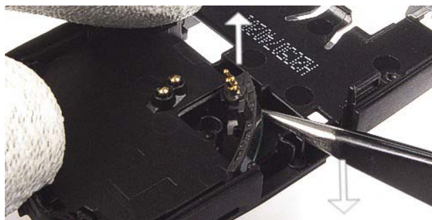
20.) Remove the Bluetooth Antenna with tweezers.
