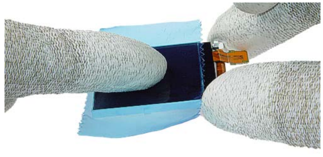
12.) Protect the LCD Module with a protective film.
