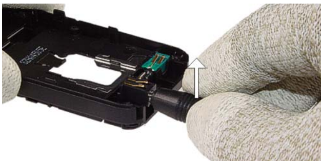
15.) Remove the DC-Jack with a DC-Plug .
