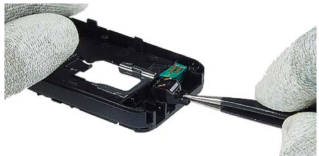
16.) Remove the Microphone with tweezers.
