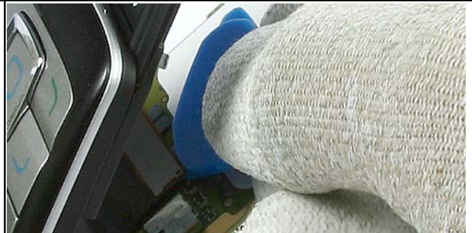
10.) Open the flex connector carefully.
