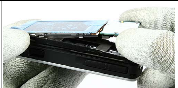
12.) Lift the UI PWB together with the LCD Module.
