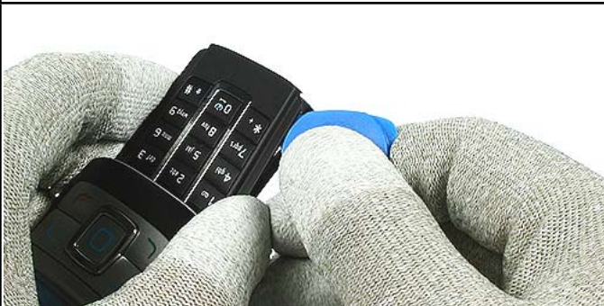
11.) Lever out the glued Keymat Assy.
