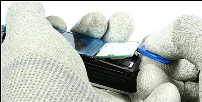
11.) Shift together the unit. Lift up the glued UI PWB Assy carefully with the SRT-6.
