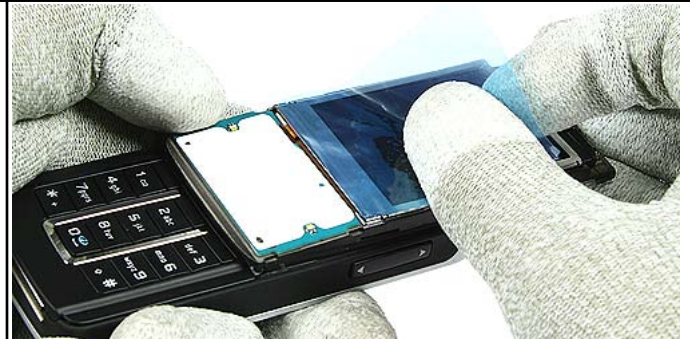
10.) Protect the LCD with a plastic film.
