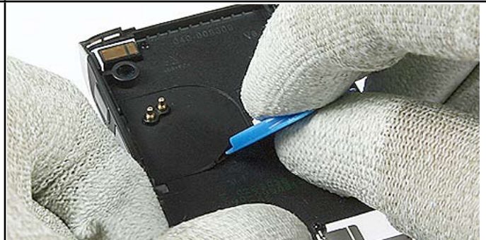
14.) Release the IHF Label with the SRT-6.
