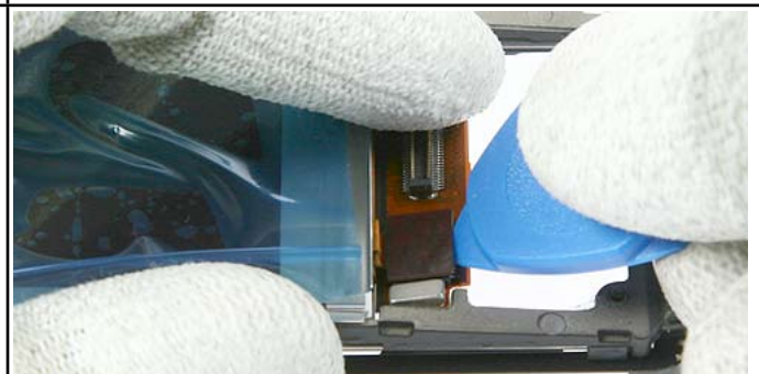
16.) Release the connector of the LCD Module carefully while fixing the flex foil. Remove the LCD Module now.
