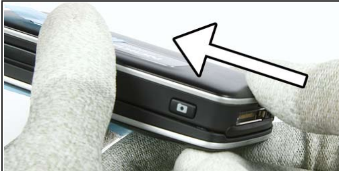
1.) Open the B-Cover by pressing it from the bottom side.
