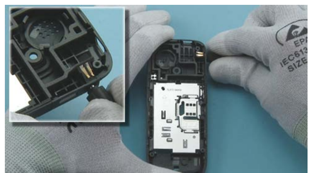
30) Release the DC JACK with the DC plug.
