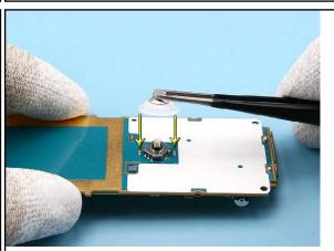
18. Use tweezers to remove the JOYSTICK HAT. Note the right position to JOYSTICK HAT when assembling the unit.
