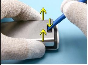
2. Press the BATTERY COVER LATCH and lift a bit the BATTERY COVER ASSEMBLY.
