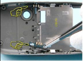
22. Gently, remove the VOLUME and FUNCTION switches using tweezers.
