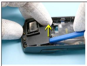
21. Remove the 1GSM ANTENNA MODULE.
