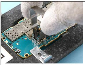
19. Unlock and remove the CAMERA MODULE with the SS-102 camera removal tool.
