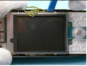
10. Unlock the UI SHIELD ASSEMBLY with the SS-93.
