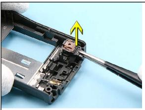
23. Remove the MICROPHONE avoiding bending the spring contacts.
