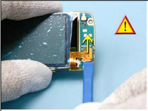
16. Carefully, open the LCD connector with the SS-93 paying attention to the surrounding components.
