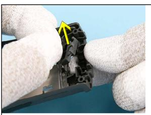
25. Remove the BATTERY COVER LATCH.
