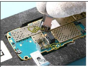
20. Note the right position of the CAMERA MODULE when assembling the unit.
