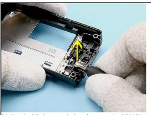
24. Use the DC-plug to unlock and remove the DC-JACK.
