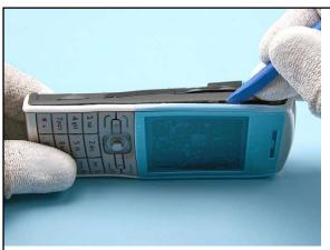
5. Slide the SS-93 along the edge to unlock the snaps.
