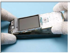
12. Remove the ENGINE MODULE from the B-COVER.
