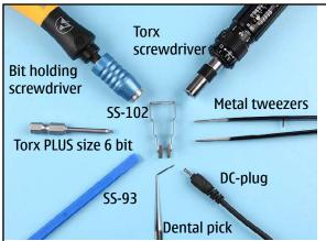
1. Needed tools: a bit holding screwdriver, a Torque screwdriver, a Torx PLUS size 6 bit, metal tweezers, a DC plug, the SS-93 opening tool, the SS-102 camera removal tool and a dental pick.
