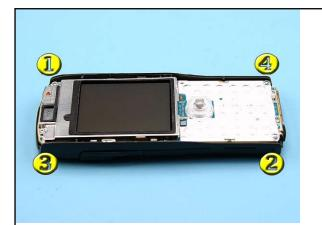
Undo the screws in the order shown and remove them. For assembly: Use the same order and a torque of 20 Ncm for re-assembly.
