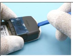
4. Unlock the A-COVER with the SS-93 starting on the top side of the phone.
