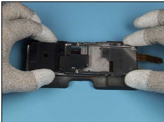
7. Position it over the flex foil assemblies, mind the guides.
