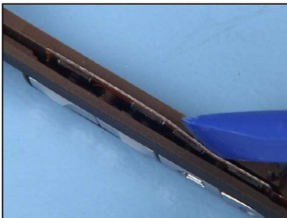
40. Carefully release the glued in CAMERA FLEX ASSEMBLY.
