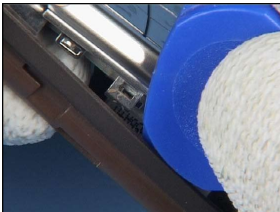
24. Shift open the assembly. Gently pry open these clips of the B-COVER with the SRT-6 in order to reach the clips of the T9 KEYMAT.
