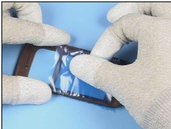
8. Protect the window from inner side.
