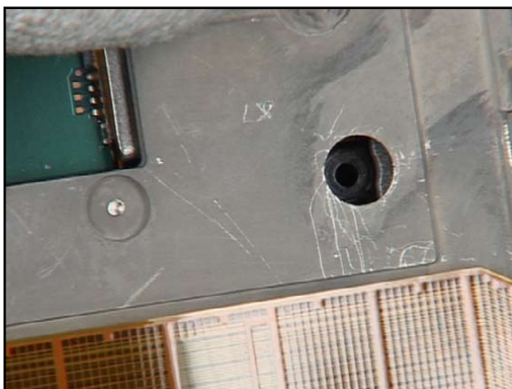
34. Bring the SLIDE MODULE ASSEMBLY into position shown to reach the hidden thread.
