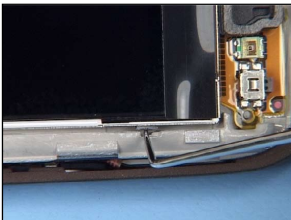
10. Carefully bend open the metal snaps of the DISPLAY HOLDER ASSEMBLY.
