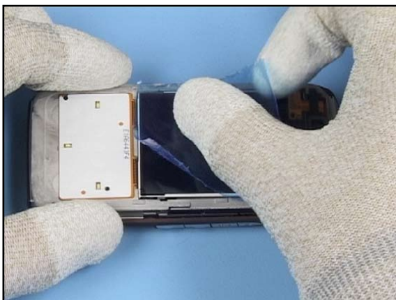
12. Cover the LCD with a protective film.
