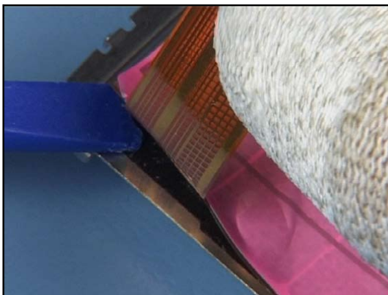
46. Peel up the T9 FLEX ASSEMBLY, beginning from the connector side.
