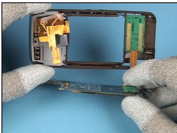
21. Close the connector of the SIM CARD MODULE.
