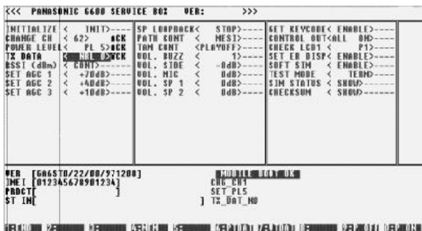
Figure 22: Channel box setup
