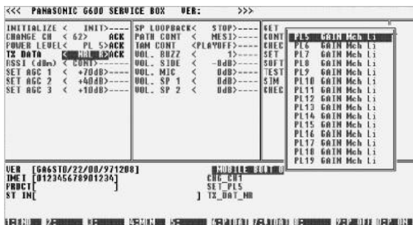
Figure 15: Power level selection 2.
