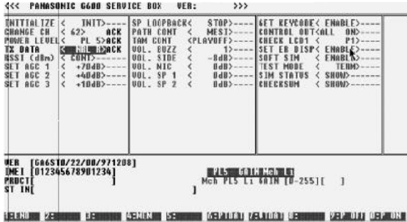
Figure 16: Power level selection 3.
