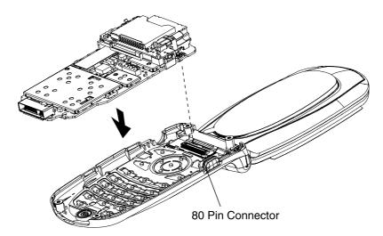
3. Reassemble the lower case assembly. Push the antenna in until it locks in position. Place the SD cover into the SD opening and rotate until snapped into place. If necessary replace the I/O cover.
