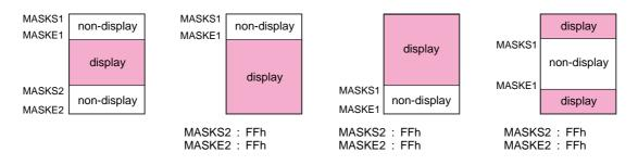
Figure 4.8: LCD Module Standby Mode
