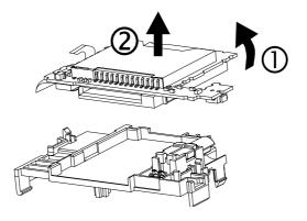
Rotate lower flex lock (2) and remove flex from bottom connector. Remove lower flex from sub PCB.
