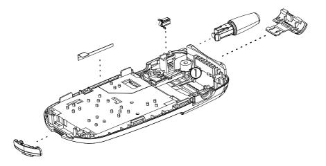
4. Place the headset jack cover in the lower case cover. Assembly the lower case with the lower cover assembly. Close the four snaps making sure that both assemblies are connected.
