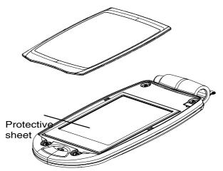
2. Place the logo panel in the recess as shown. Ensure that the logo panel is seated correctly. Press and hold the adhesive areas (at each end) with moderate (not excessive) force to the upper cover for ten seconds
