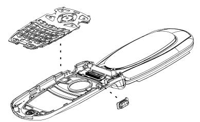
2. Place the upper housing into the lower cover assembly. Connect the 80 pin connector halves by using the thumb and forefingers to apply force to the exterior areas directly over the connector. A snap should be heard or felt to insure a secure connection.
