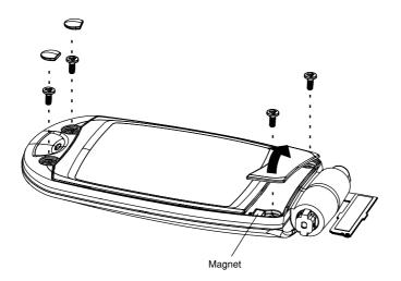
3. Separate the upper cover and upper case using a plastic strip (of credit card thickness). **Note:** There are two snaps on both sides of the phone.
