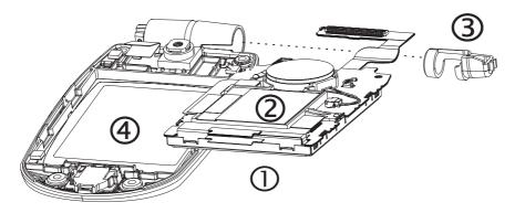
4. Attach the PCB connector into the receiver (1) and (2). Attach the camera connector to the connector on the PCB (3). Caution: Damage to the flex circuit portion of the upper flex PCB is NOT repairable. The flex circuit may be easily stretched or cut during this operation, causing a small tear which can grow with use and render the circuit unusable. Handle this assembly with care to avoid damage.
