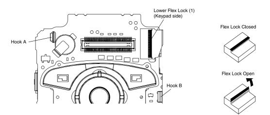
2. Turn main PCB over if necessary pivot (1) to release chassis from PCB. Lift up (2) and remove.
