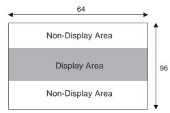
Figure 4.9: Sub-LCD Dimensions
