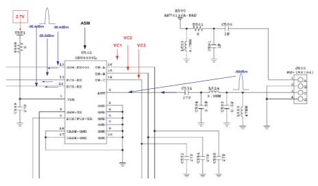
Figure 8.1: Front-end Module (U502), receive-path signals
