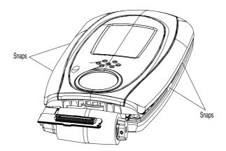
4. Gently press down (1) and slide the flex circuit towards the top of the phone (2). This will remove the flex connection from the brackets. Gently lift up camera connection flex (3).
