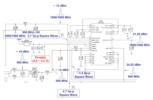
Figure 8.5: Tx SAW filter (UFL507) and Power Amplifier (U503), transmit-path signals
