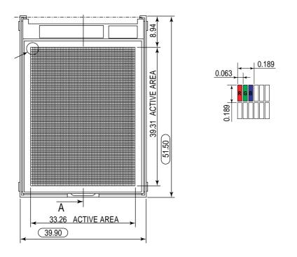
Figure 4.7: Main LCD Dimensions
