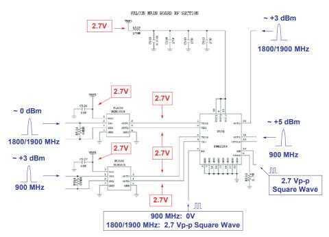
Figure 8.4: 3rd Harmonic (H3) filters (FL500 and FL501) and Limiter Amplifier (U501), transmit-path signals
