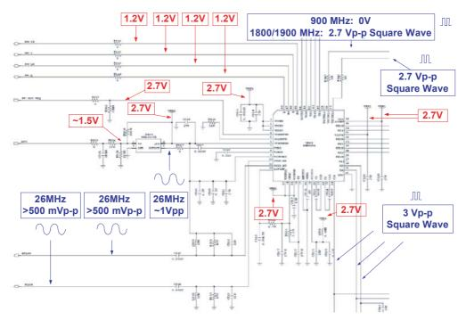
Figure 8.3: Transceiver IC (U500) and VCTCXO (Y500), clock and control signals
