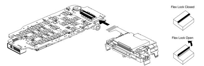
3. Carefully rotate the SD PCB assembly to the opposite side of the main PCB and align the three tabs. Take care not to damage the SD flex during this step. Press the SD PCB assembly and the main PCB together. Make sure that the two locking hooks properly engage.
