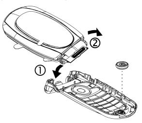
3. 1) Insert hinge holder into the lower cover in the direction shown. 2) Gently lower the other side of the hinge holder into the lower cover. Insert the retaining screw and torque to 1.3 KGF-CM using a #3ULR0 Trident screwdriver tip.
