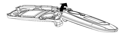
2. Using a strip of plastic (of credit card thickness) gently lift up and remove the logo panel. Remove the two screw caps. Use a Trident screwdriver to remove the four screws securing the logo panel. Retain the screws for reassembly.
