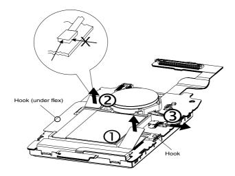
2. Lift and remove sub LCD module.
