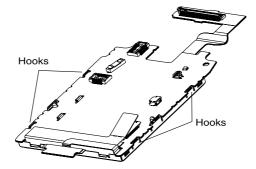
4. Remove main LCD module.
