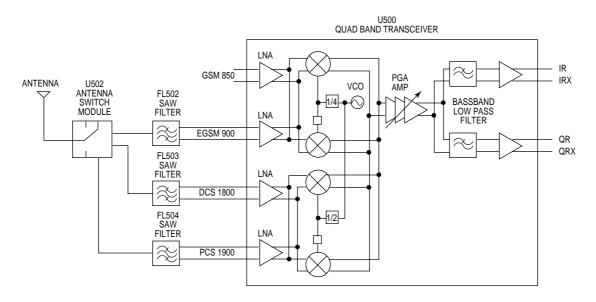
Figure 4.4: Receiver Block Diagram
