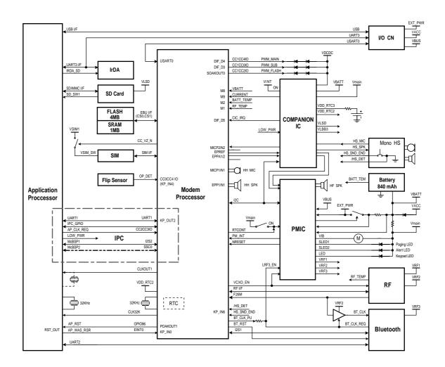
Figure 4.5: Baseband Block Diagram
