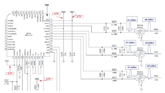
Figure 8.2: Transceiver IC (U500) and Rx band-pass filters (FL502, FL503, and FL504), receive-path signals
