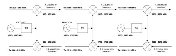
Figure 4.2: Frequency Plan
