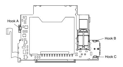
4. Pivot (1), lift (2) and remove sub PCB.
