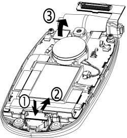
5. Lift bottom end of flex PCB board and slide right until board clears the camera and is free from the upper cover. The hinge pivot will exit the hinge compartment while removing the flex PCB board.
