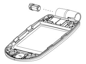
2. 1) Rotate and align the hinge pivot with the open area facing upward and carefully insert into the main area of the lower cover assembly, taking care to tilt the upper housing assembly without causing damage to the flex circuit during reassembly. 2) Push down gently until the upper housing assembly is full engaged into the lower cover. Insert microphone.
