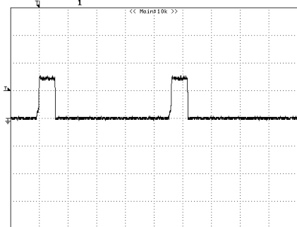
4 C327 EGSM/DCS/PCS (Talking) (CH1=1V, 1ms/div)
