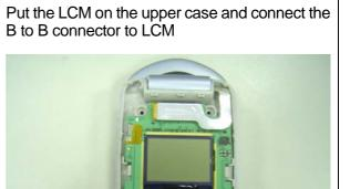
Insert and tighten the 4 screws  $(11 \pm 2 \text{ cNm})$
