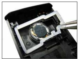
Use the tweezers to remove the loudspeaker out of its proper position, without touching the contacts.
