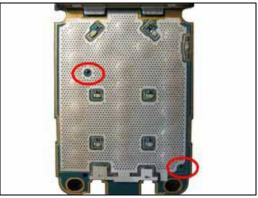
Attach two new conductive gaskets.
