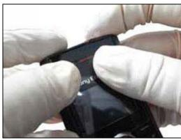
Snap the side hooks to frame housing.
