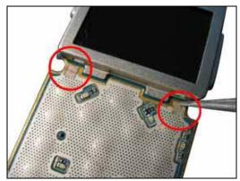
Use the tweezers to peel off the dome foil from the PCBA
