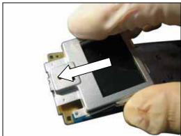
Put the LCM Metal Frame in the guiding hole for the PCBA.
