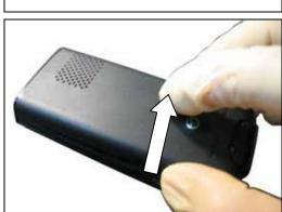
Lift and remove the Battery Cover
