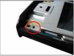
Press the PCBA down till snapped to the Frame Housing.
