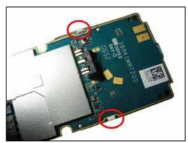
Release the LCM Metal Frame
