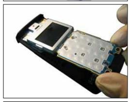
MAKE SURE THAT GUIDE PIN IS NOT DAMAGED DURING THIS PROCEDURE!
