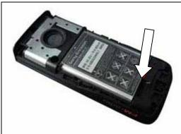
Position the battery cover into the frame housing at the top and put down the two parts together.
