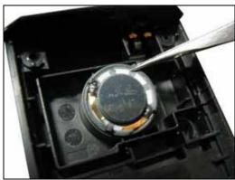
Remove the protective tape on the loudspeaker.
