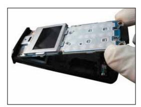
Make sure that the guide pin is inserted into guide holes of PCBA and metal carrier.
