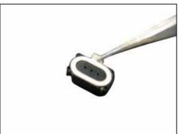
Use the tweezers to place the new earphone in is proper position and press gently, without touching the contacts.
