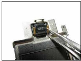
CLEAN THE CORRESPONDING SURFACE OF METAL CARRIER TO REMOVE ADHESIVE.
