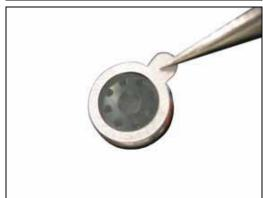
Use the tweezers to place a new loudspeaker in its proper position and press gently, guide pin into recession, without touching the contacts, until it reaches the bottom of the cavity.
