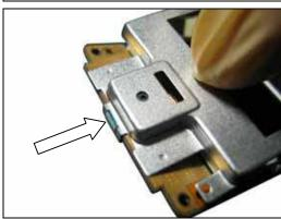
Press down on the bottom corners of LCM Metal Frame to snap two hooks onto the LCM.
