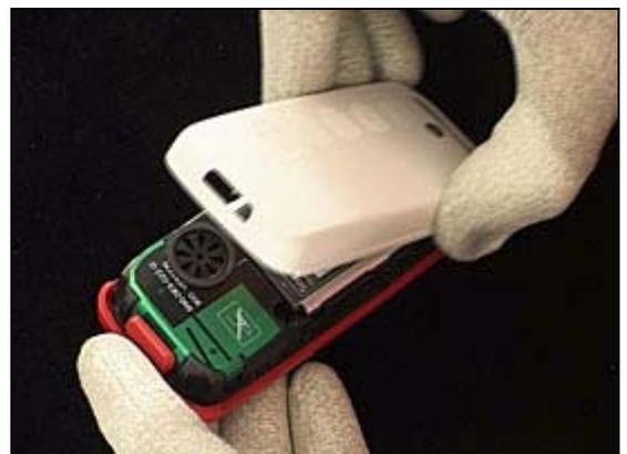
Press on both sides at the top until the *rear cover* is securely snapped to the frame cabinet.
