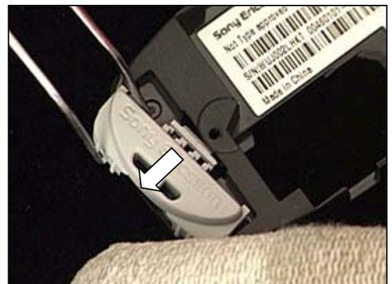
Put the *strap holder* in position and push it onto the frame cabinet ...
