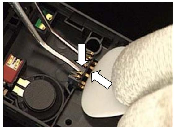
until the *battery connector* drops down into its proper position.
