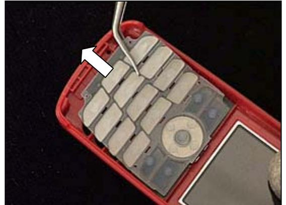
Place the *keypad* inside the front cover and press with your fingers to attach it to the front cover.
