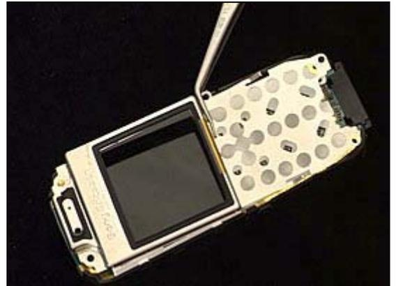
Place the *light guide* on the lower part of the metal carrier.
