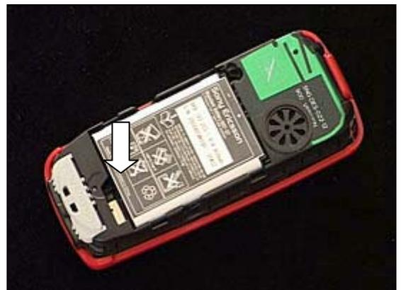
Position the *rear cover* into the frame cabinet at the bottom and put the two parts together.
