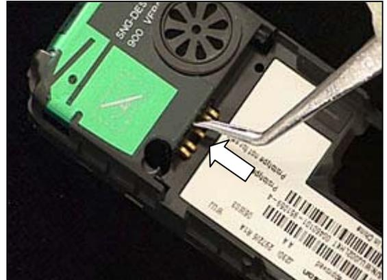
until the *battery connector* falls out of the frame cabinet.
