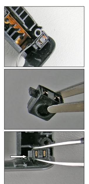
Use a pair of tweezers to assembly the Microphone Assy. The knob of the Microphone Assy should be upwards.
