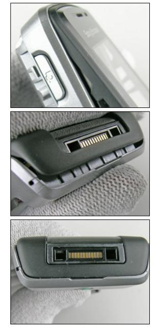
Press it in place. Start at the top and press down to the bottom. When finish there should be no gap between the Front Cover Assy and the Frame Sub-Assy
