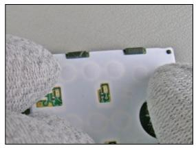
Use a dentist hook to release the Domesheet Assy from the UI Module Frame and simultaneously press under the Domesheet Assy.
