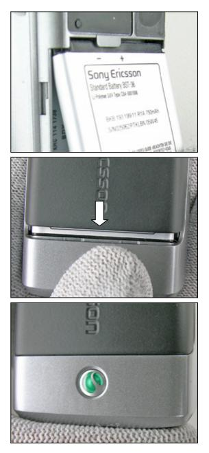
Place the battery cover on the B-cover. Press it down to secure it.
