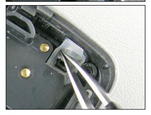
Use the pair of tweezers to assemble the Power Key Assy. Place the knob in the notch.
