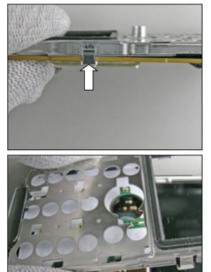
Grab the Metal at the top and carefully push it upwards and remove the Metal Frame Assembly.
