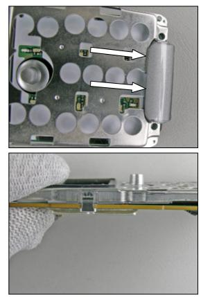
Press the Metal Frame Assembly together with the PWB Assy.
