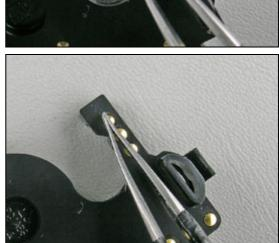
Use the pair of tweezers to assemble the Pogo Pins in the corresponding holes.
