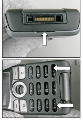
Grab the Front Cover Assy and carefully remove it from the Frame Sub-Assy.
