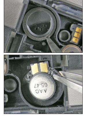
Use the pair of tweezers to assemble the Speaker.
