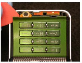
Carefully peel the keypad off the hinge assembly.
