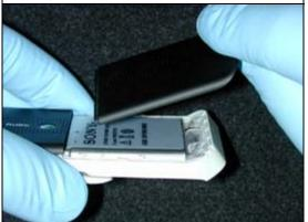
Lift the end of the battery cover to remove it.
