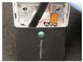
Push the pry tool into the seam and toward the left side of the cover so that latch holding the left corner of the cover releases.
