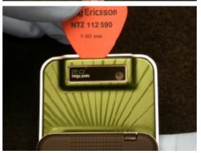
Pull the lifted end of the camera cover as shown to remove the camera cover.
