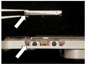
Work the volume key into its opening so that the features at each end of the volume key mate with the features of the frame as shown.
