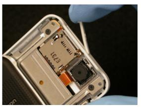
Rotate the memory stick cover down to free the inside latch from the peg on the frame.
