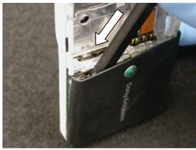
Lift up on the rear cover to release the middle and right side latches.
