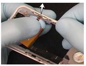
Push the camera out of its cavity.
