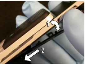
Separate the navigation keypad from the front cover.
