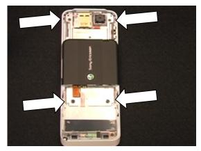
Use the magnetism of the wrench to pull the bottom screws up through the hole in the hinge.
