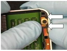
Snap the tab on one side of the frame in the slot on the hinge.
