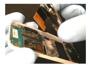
Lift the hinge assembly from the rear frame.
