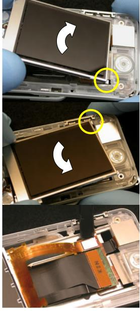
Once free, lift the LCD assembly out of the way and detach its flex connection using a pry tool.
