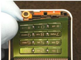
Align the tabs and notches on the keypad with the tabs and holes indicated on the hinge assembly.
