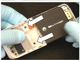
While holding the hinge in the partially closed position, remove the screws.
