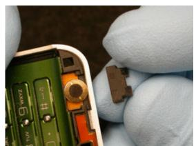
Press the gasket over the microphone as shown.
