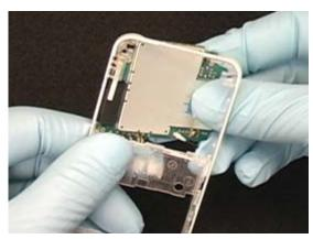
Position the coaxial cable so that it passes through the hole formed between the notch in the circuit board and the rear frame.
