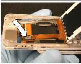
Fold the LCD so that it lays over its cavity.
