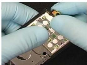
Pull the vibrator pads through the slot in the hinge.
