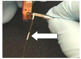
Insert the connector into the slot of the tool, and then snap the connector onto the antenna.
