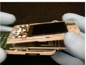
Lay the front of the phone loosely on top of the hinge
