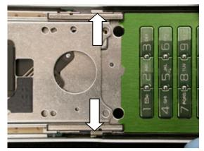
Insert tweezers or a small screwdriver under one of the metal clips and twist toward the center of the phone to release the latch.
