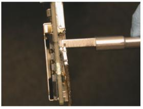
Pull the connector directly away from the PC board.
