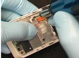
Slide the hinge partially closed until the remaining 2 screws are visible.
