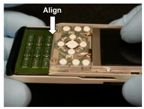
Lift the bottom edge of the phone's upper half approximately 10-15 mm.
