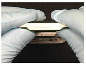
Open the memory stick cover and ensure the memory stick housing correctly lines up with the opening. If it does not, remove the camera cover and reposition the memory stick housing.
