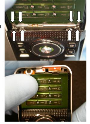
Apply pressure over the surface of the keypad so that a good bond to the hinge assembly occurs.
