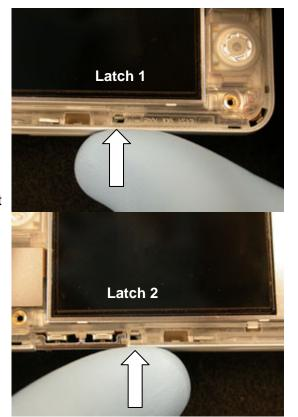
One at a time, press inward on the side of the front frame at each of the latch locations to release the latches.
