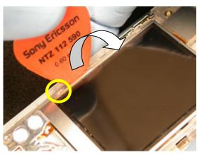
Insert the tip of the plectrum between the right side of the LCD and the front frame.
