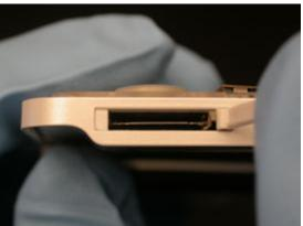
While holding the camera cover in place, turn the phone over and bend the two metal tabs toward the center.
