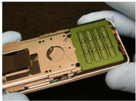
Press the end of the hinge assembly that contains the microphone into the rear frame.
