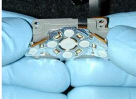
Insert the top of the navigation keypad/ speaker box into the cavity on the frame with the keypad in front of the frame and the speaker box in back of the frame.
