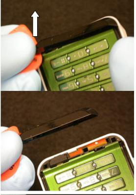
Remove the microphone gasket using your fingers.
