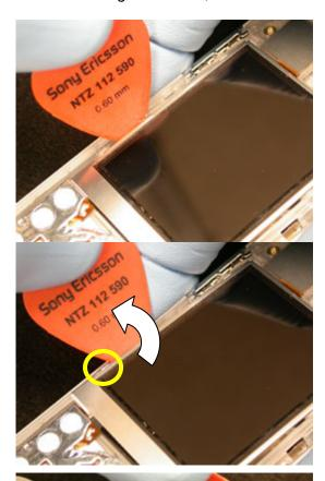
Rotate the plectrum away for the LCD to release the lower left side retention feature.
