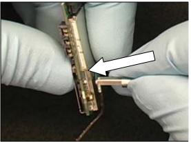
Rotate the coax cable so that it is oriented to the circuit board as shown.
