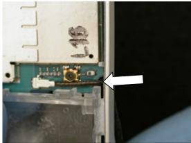
Work the side of the circuit board opposite the system connector into the rear frame by pulling the portion of the rear frame indicated away for the circuit board so that the two snaps clear the board's edge.
