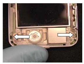
Use a rounded tipped tweezers to bend the metal tabs up.
