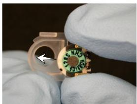
Insert the receiver/gasket assembly into the cavity on the front frame.
