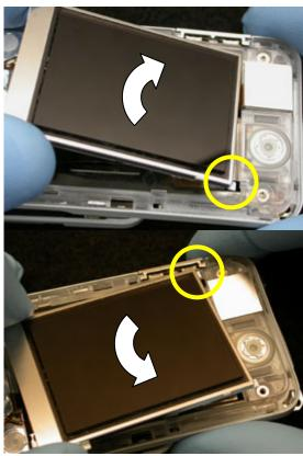
Once free, lift the LCD assembly out of the way and detach its flex connection using a pry tool.
