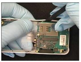
Lift the circuit board, coaxial cable, and antenna as one unit from the rear frame.
