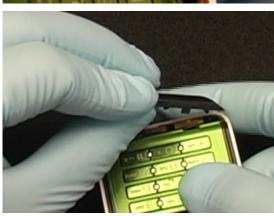
Push down on the cover to snap all the tabs into place.
