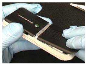
Push the bottom edge of the battery cover downward and towards the top of the phone to get the battery cover to slide into place.
