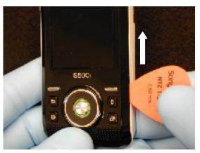
Slide the plectrum around the top corner to release the upper right corner latch.
