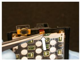
Orient the vibrator so that its spring fingers are toward the vibrator contact pads and insert the vibrator into its cavity.
