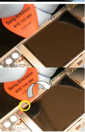
Rotate the plectrum towards the LCD to insert the lower left side retention feature into its slot in the front frame.
