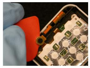
Hold the flex with one finger while working the microphone pins out of the holes.
