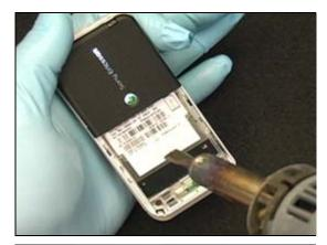
Use rounded tip tweezers to start the peeling up of the label.
