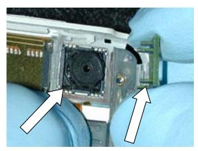
Insert the pegs into the slots and press the tool completely onto the camera.
