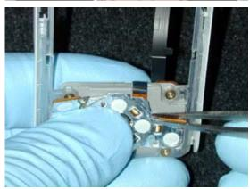
Push the bottom of the speaker box from the frame.
