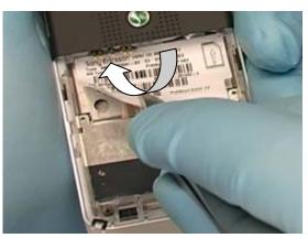
Push the label down into the battery cavity and make sure the Liquid Intrusion Indicator shows through the square hole.
