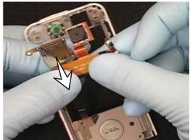
Fold the top corners of the dome foil a small amount off the speaker box.
