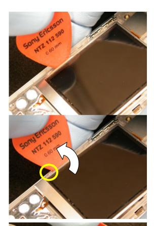
Insert the tip of the plectrum between the right side of the LCD and the front frame.
