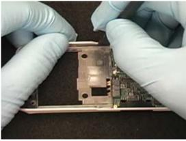
Insert the peg of the power key into the hole on the rear frame and press it into place
