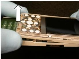
With the bottom edge the phone's upper half lifted, locate the two side latches holding the front frame on the hinge.
