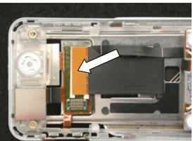
Orient the LCD as shown and plug the LCD's flex into the bonzer flex.
