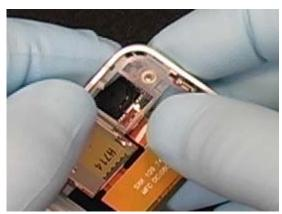
Insert the volume switches into their cavity.
