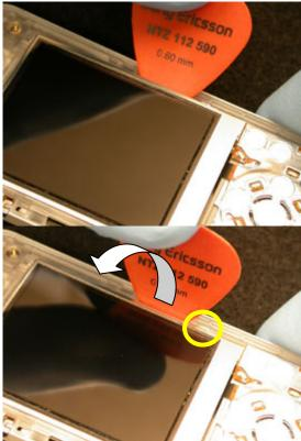
Rotate the plectrum towards the LCD to insert the lower right side retention feature into its slot in the front frame.
