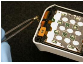
Insert the pins into the holes.
