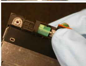
Plug the keypad flex to the hinge flex.
