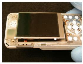
Insert the upper two LCD retention features into their slots in the front frame by wiggling to LCD to the right and then the left.
