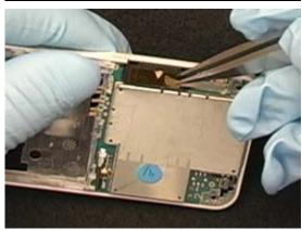
Grip the middle of the antenna assembly and rotate it away from the circuit board to free the antenna from the rear frame
