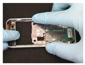
Push the coaxial cable down into the slot of the frame using a pry tool.
