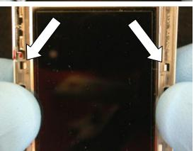
Press in on the front frame at two side latches to get the hinge and front frame latched together.
