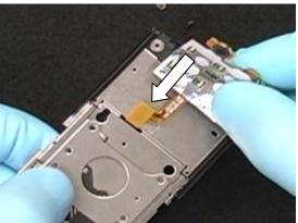
Using the features around the hinge assembly's keypad area for alignment, place the keypad flex on the hinge.
