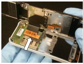
Lay the hinge assembly on top of the frame
