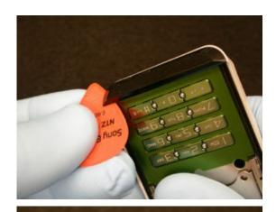
Using the plectrum, lift up of the left end of the chin cover to get the chin cover to unsnap from the rear frame.
