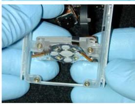
Fold the top corners of the navigation keypad down onto the frame.
