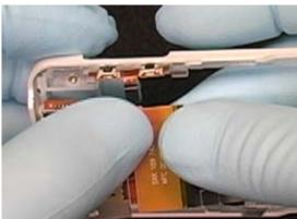
Place the memory stick holder portion of the flex within its retaining features in the front frame.
