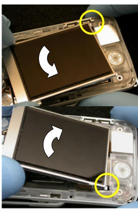
Insert the tip of the plectrum between the left side of the LCD assembly and the front frame.
