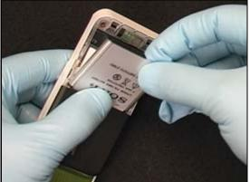
Pull the battery out of the battery cavity.
