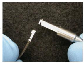
Using the tool, snap the connector onto the PC board.
