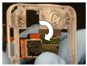
Lift the portion of the flex containing the memory stick holder from the front frame.
