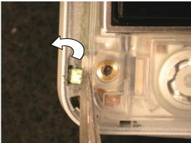
Insert a plectrum between the camera cover and the frame in the location shown to pry the cover up.
