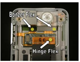
Plug the hinge flex into the corresponding bonzer flex connection.
