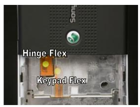
Install the microphone in the new keypad flex by performing the installation portion of the Microphone Replacement procedure
