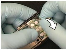
Pull the flex connector through the hole in the hinge.
