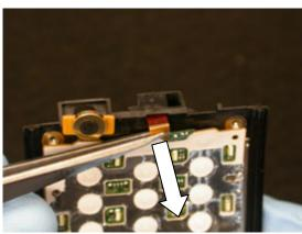
Peel the dome foil off the hinge.
