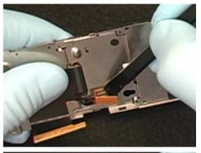
Use a pry tool to remove the vibrator.
