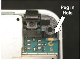
Install the Bluetooth tape using tweezers. Align the tape with the inside edge of the system connector and leave two holes exposed.
