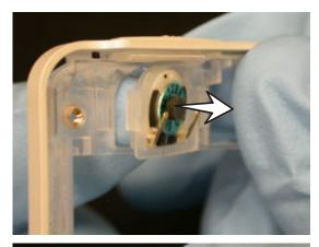
Separate the receiver and the gasket.
