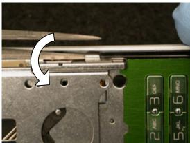
Insert tweezers or a small screwdriver under the other metal clip and twist toward the center of the phone to release the latch.
