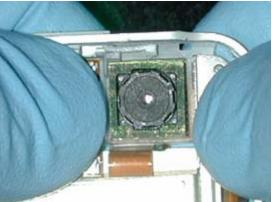
Remove the tool and the camera from the socket.
