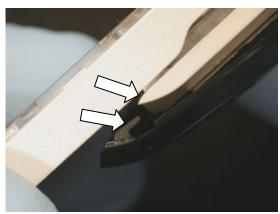
Squeeze the sides and top of the phone to snap the front cover into place.
