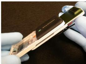
Rotate the upper end of the front cover away from the phone just enough that the side latches are clear of the frame
