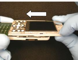
Holding the front frame and hinge assembly at the top, slide the phone closed.
