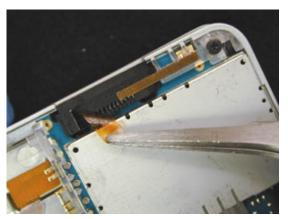
Remove the Bluetooth antenna from the rear frame by sliding it toward the edge of the frame.
