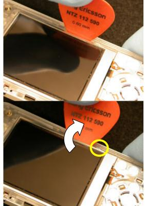
Insert the tip of the plectrum between the right side of the LCD and the front frame.
