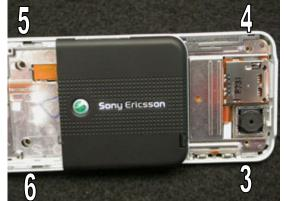
Push the hinge open and install the remaining four screws.
