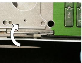
Lift the "non-keypad" end of the hinge assembly away from the rear frame.
