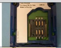
2. Check whether the antenna connector on the PCB is damaged, dirty, or oxidized. Clean it if necessary.
