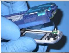
2. Remove the microphone grommet and microphone from the microphone cavity at the bottom of the front cover. Set the microphone aside for safekeeping and dispose of the microphone grommet since it cannot be reused once the phone has been opened (screws removed).
