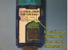
7. To remove the phone board and avoid damaging the label, slightly lift the top corner of the phone board that is near the speaker port.
