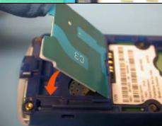
8. Apply pressure over the entire surface of the antenna assembly to ensure a good adhesive bond to the back frame.
