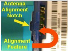
7. Once aligned, rotate the antenna assembly down into place on the back frame. Make sure that the antenna assembly's board connection fits securely into the appropriate opening at the top right side of the back frame.
