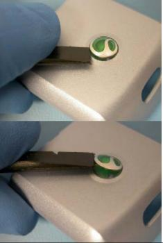
3. Remove the backing from a new SEMC icon and place the icon in the corresponding cavity in the antenna cover.
