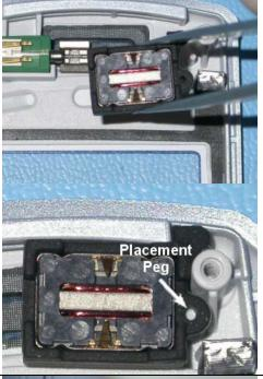
21. Place the keypad PCB assembly into the new front cover with the dome foil side down and the contacts toward the bottom of the phone.
