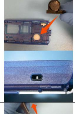
8. Using tweezers, gently pull the volume switch out of the old back frame.
