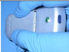
2. Remove the battery by inserting a pry tool underneath the tab at the bottom of the battery and rotating the pry tool so that the flat edge of the tool moves into a vertical orientation.
