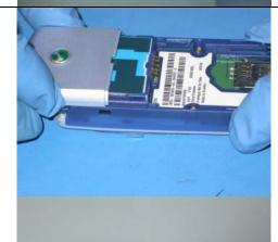
6. Starting with the top of the battery, place the battery, label-side up, into the battery cavity. Make sure that the tabs at the top of the battery fit into the corresponding slots in the top of the battery cavity.
