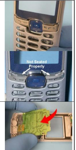
5. Place the keypad PCB assembly into the front cover with the dome foil side down and the contacts toward the bottom of the phone.
