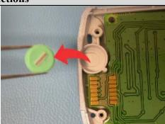
2. Place a new microphone into the old microphone grommet.
