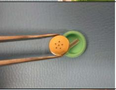
3. Place the microphone assembly into the microphone cavity at the bottom of the front cover, with the contact side up (as shown).
