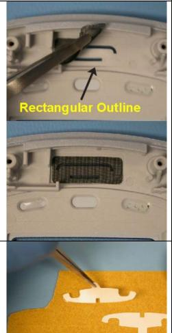
5. Remove an inlay adhesive film/backing assembly from the large strip of backing containing the adhesive film/backing assemblies.
