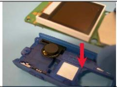
2. Place the front cover and the back frame assembly together.
