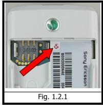
On the pictures below you will see the different between a sticker that has been in contact with liquid (Fig. 1.2.3) and with one that hasn't (Fig. 1.2.2).
