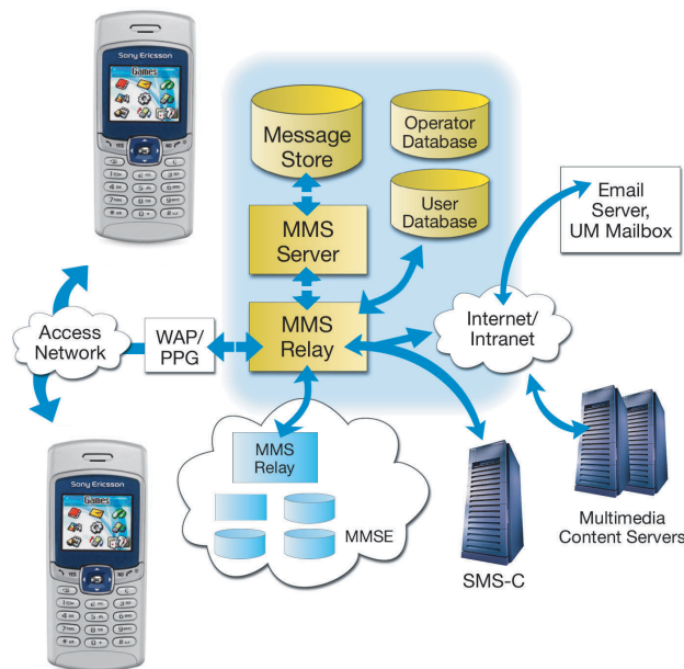
Figure 3. The architecture of MMS
