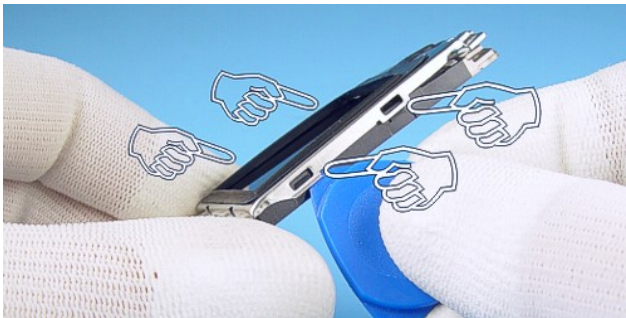
12) Unlock the clips with SRT-6 on both sides of the Display Shield .
