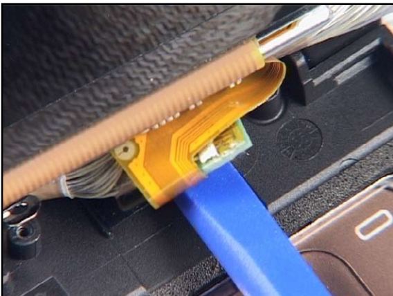
21. ...and, using SS-93, carefully pull out the display connector from the UPPER A-COVER.
