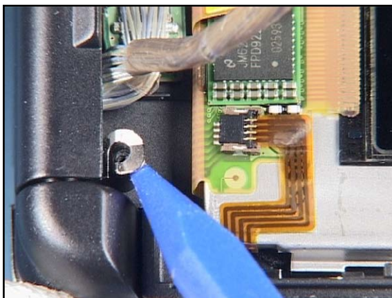
10. Lift the metal tab as shown...
