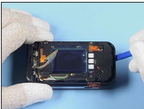
16. Unlock the UPPER C-COVER ASSY using the SS-93...
