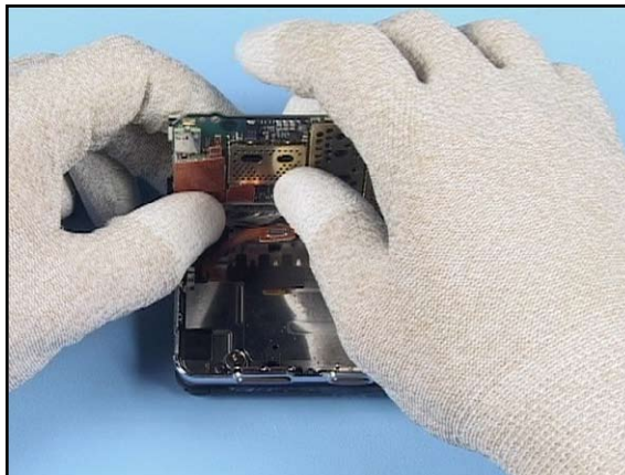
8. Lift up the PWB and hold it as shown...
