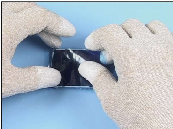
22. Cover the display surface with the protective film.
