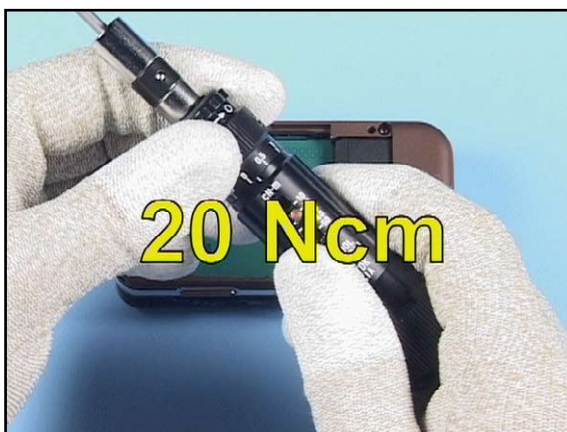
18. Set the torque driver to the torque of 20 Newton centimeter.
