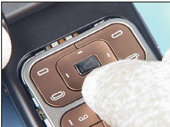
22. Place the KEYMAT onto the LOWER A-COVER...
