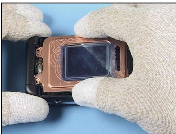
18. Align the SECOND DISPLAY FRAME ASSY with the UPPER C-COVER.
