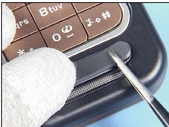
24. Using a new A-COVER ASSY fit the new BUMPER.
