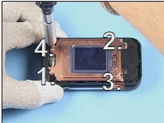
22. Tighten the screws to the correct torque in the order shown.
