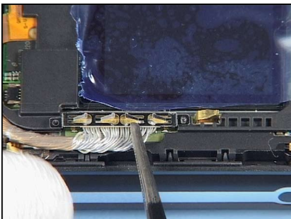
15. Place the COAX GROUNDING SPRING over the connector.
