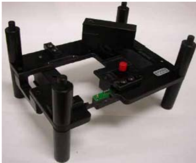
Figure 7.2. : PCB Repair Jig
