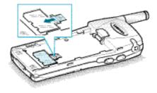
6. Place the battery back on the phone. Slide the battery up towards the catch until it locks into place. Make sure that the battery is properly installed before switching on the power.
