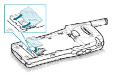
Note: If you need to remove the SIM card, carefully slide the SIM card lock back and take the card out of the holder.
