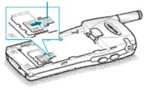
4. Insert the SIM card under the two tabs, ensuring that the cut corner faces towards the bottom of the phone and the gold contacts of the card face into the phone.
