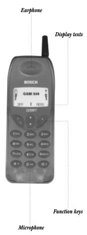
The function keys have different functions according to whether you are in standby or conversation mode. The display text above the key will inform you of the actual function of the key at any time.
