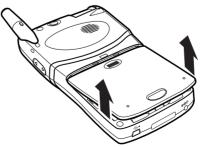
5. Hold both sides of the battery, and then lift and remove the battery.
