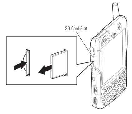
Push the card slot protector until it clicks, and then release your finger to cause the protector to be ejected. Slowly pull the ejected protector out of the slot. **2.** Hold the card so that its top surface and the touch screen face the same direction, and then insert the card into the SD card slot. Push the card until it clicks.
