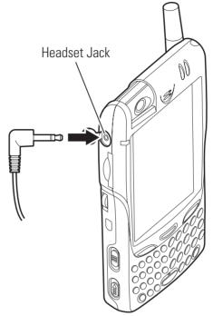
**Note:** Insert the headset plug into the jack as far as it goes. Incomplete connection of the headset plug can result in abnormal sounds.
