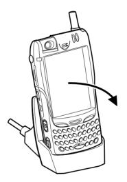
**Note:** After the device has been mounted onto the USB cradle, the vibrating device (if switched on) does not function when a call is received.
