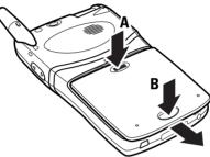
**2.** Slide the battery cover until the cover comes out of the guides, and then lift and remove the cover.
