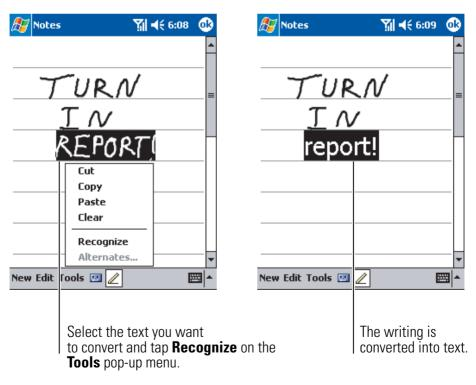
If the conversion is incorrect, you can select different words from a list of alternates or return to the original writing. To do so, tap and hold the incorrect word (tap one word at a time). On the pop-up menu, tap **Alternates**. A menu with a list of alternate words appears. Tap the word you want to use or tap the writing at the top of the menu to return to the original writing.
