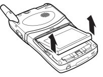
Note: If the battery is removed with the device on, data will be lost.
