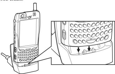
**2.** Tilt the device in the direction of the arrow so that its tab hole is aligned with the tab on the cradle.
