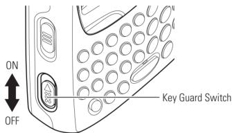
Turning on the Key Guard switch (up position) places the device into the following status:
