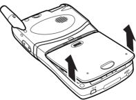
**3.** Hold the main battery with the label surface facing upward, and then install the battery so that the grooves at both sides mate.
