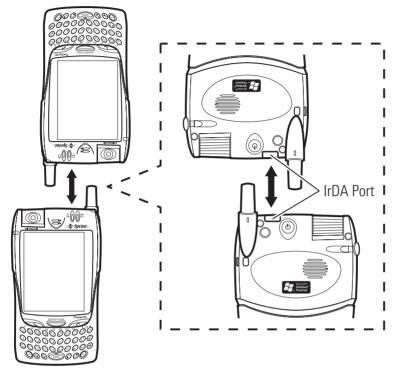
Be careful that the IrDA ports line up within 15 degrees in the horizontal and vertical directions and that the distance between the two devices is less than 70 cm (27.5 inches).
