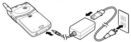
The LED for Charging lights amber while charging is being performed. The LED turns green when charging is completed. For more information about the LED for Charging, see "LEDs" on page 29.
