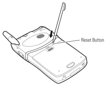
**Note:** Resetting the device causes data not yet saved to be lost. Data that has been saved will not be lost through this operation.
