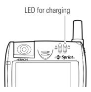
It takes approximately three hours to finish charging a battery that has only enough power for data backup, but not enough for operation. **Note:** Charge the battery at an ambient temperature in the range from 0°C to 35°C (32°F to 95°F). Depending on the operating conditions of the device, charging may be interrupted even when the ambient temperature is lower than 35°C (95°F).
