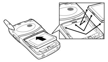
**4.** Using the stylus, shift the Full Reset switch upward to unlock it. (The switch is locked before the device is shipped.)
