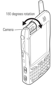
**Note:** If the lens is dirtied with fingerprints, oil, or grease, clean it with a soft cloth before taking pictures.
