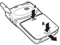
**4.** Slide the battery cover until the cover comes out of the guides, and then lift and remove the cover.
